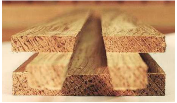
▲ Pic.5 Some of the rails are complex routing operations, with tenons at the end. This is the outer frame middle rail (E)
